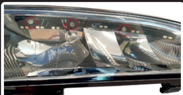
The emitter is fastened through the backside of the lamp, using the included screws.
